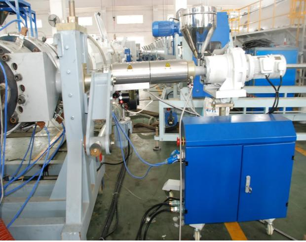
Type:30-25 Maximum output:1.5kg/h Weight :200kg Material of screw: 38CrMoAlA Treatment: Nitriding processing, depth0.5~0.7mm polishing Motor :1.1kw Inverter: Danfoss With stainless steel hopper For the computer control system for all of our extruders, Liansu uses Simens HMC-II 300 series, with 10 inch key screen.
