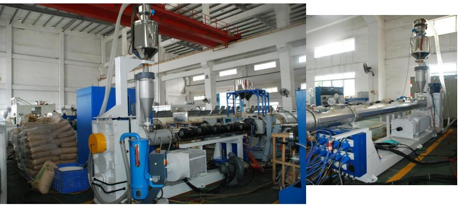
Main driving motor : 200kw DC motor Auto feeding unit(with dryer): supplier: Taiwan Shini Electric heating power :6 kw
