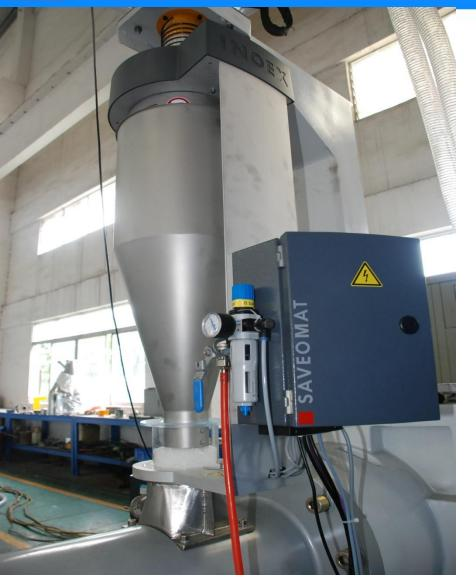
Saveomat IGS.M1 Gravity monitoring system, it is directly imported from Germany, the purpose is for better control of thickness of pipes and stabile feeding of materials through changing the screw rotate speed and hauling speed.
