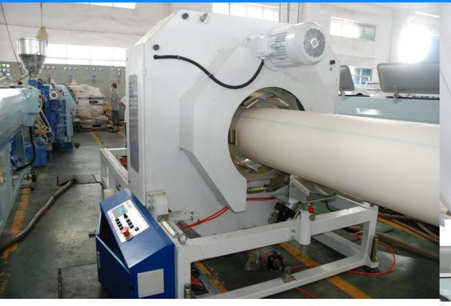
Type: Gear transmission knife in and out by screw rod rotating cutting Clamping mode: 6 connecting rods auto clamping Moving :Driven by screw rod Moving method of work table: Cylinder following Dimenstion:5650(length)  $\times$  1750(width)  $\times$  1950(height)mm
