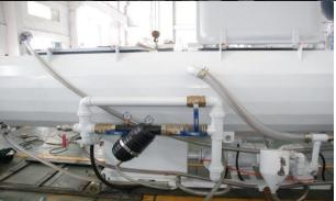
Fore & back movable distance:1200mm Water level controlled by floating ball switch; Water temperature: controlled by thermo regulating drainage valve With reliable PE filter
