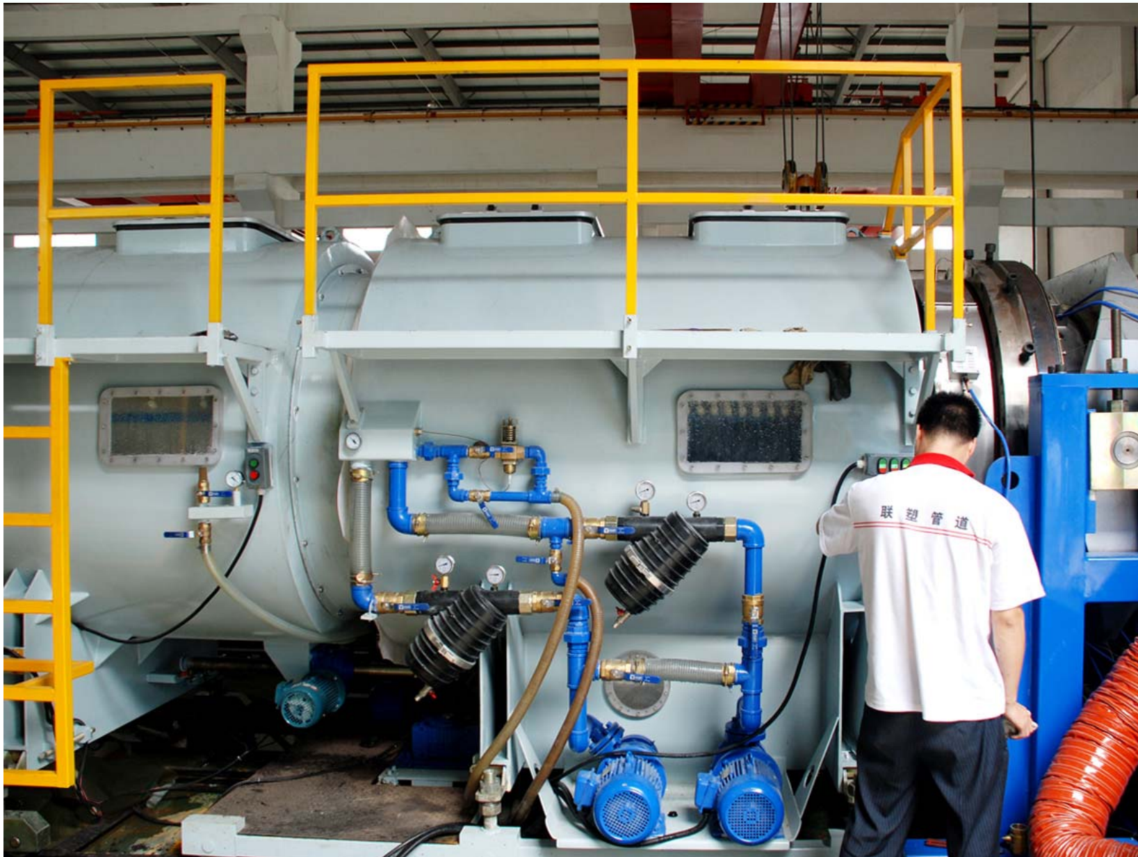
The 2 meter vacuum tank with calibrator under commissioning.
