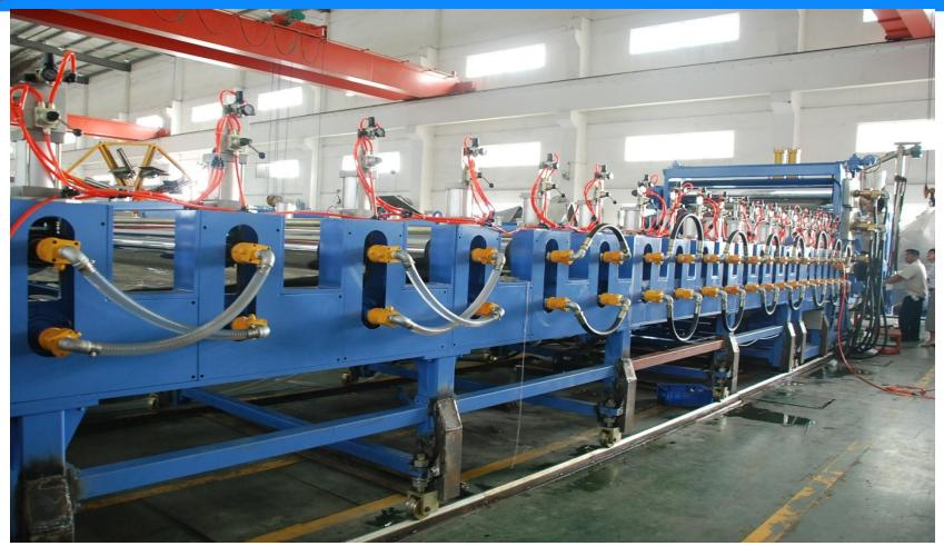
Composed of 12pairs of cooling calibration steel roller
