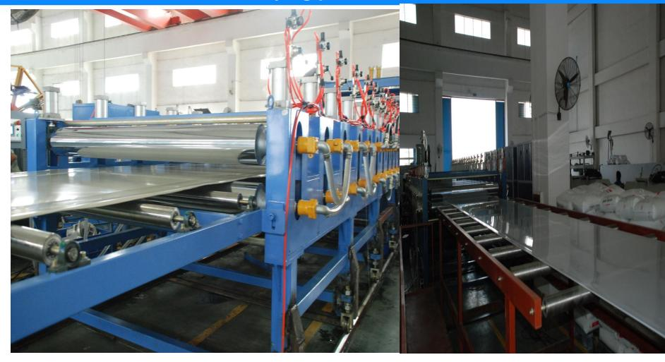
Conveying roller: Ø63~Ø74mm, chrome plated steel roller or stainless steel
