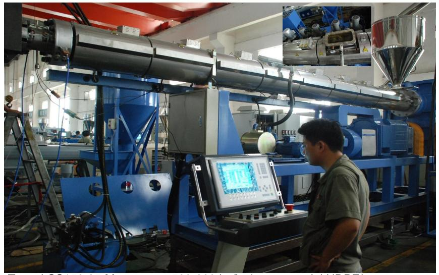
Type: LSS150-35 Max output :500-600 kg/h (new material HDPE)
