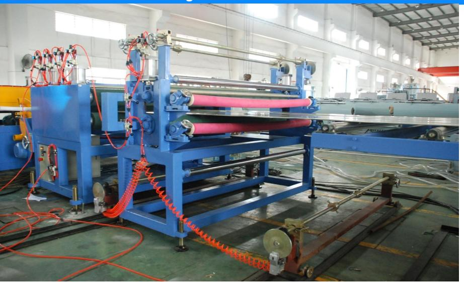
Silica roller diameter:Φ190mm,2pcs pneumatic brake device, conical surface expanding shaft Bending rubber roller flattening Φ100mm,2pcs
