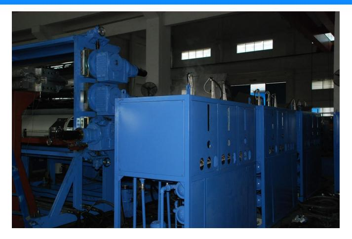
Hot oil exchanger :3sets Tri-roller each with oil circulation temp control system
