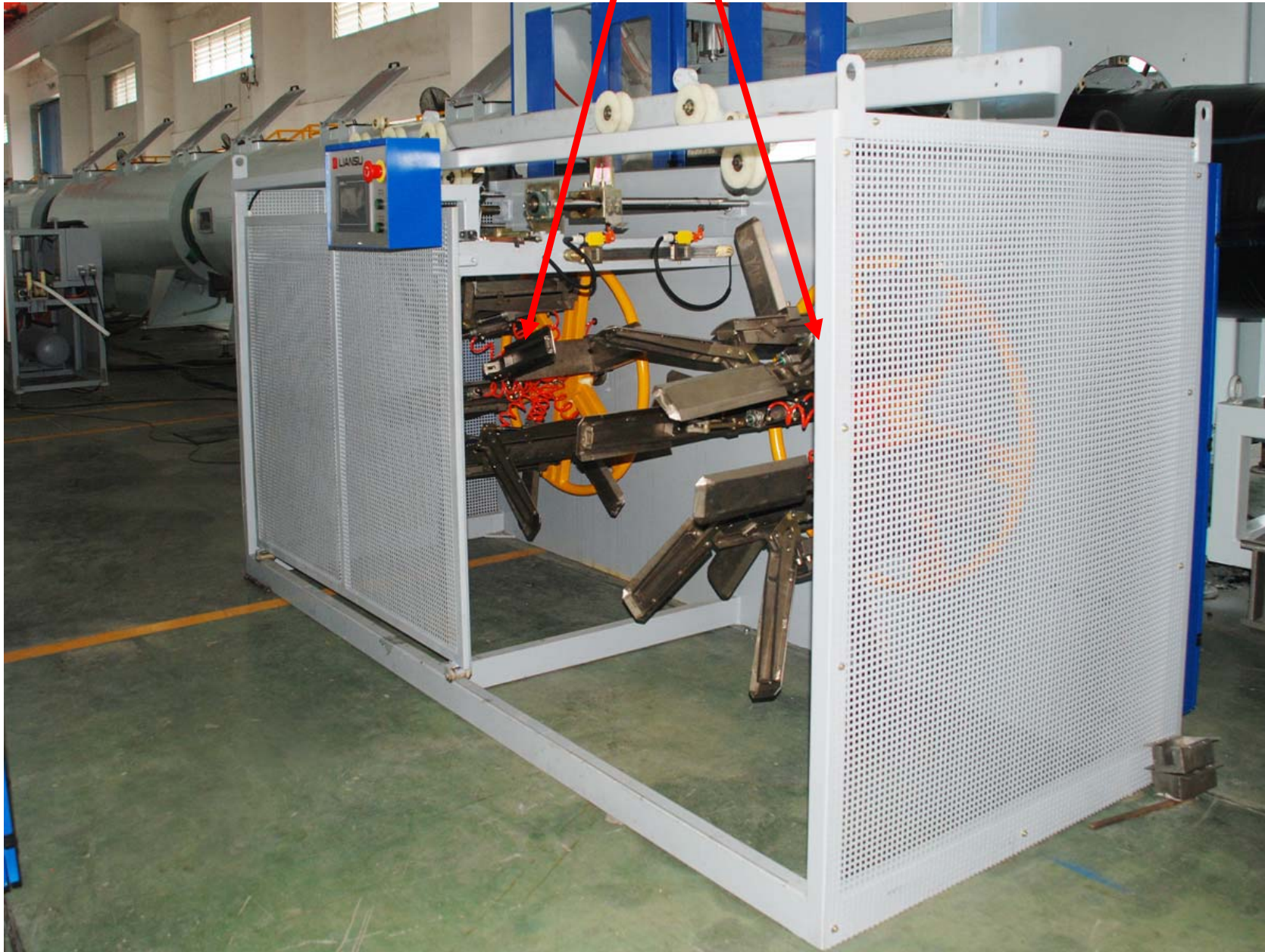
Double roller winding station design
