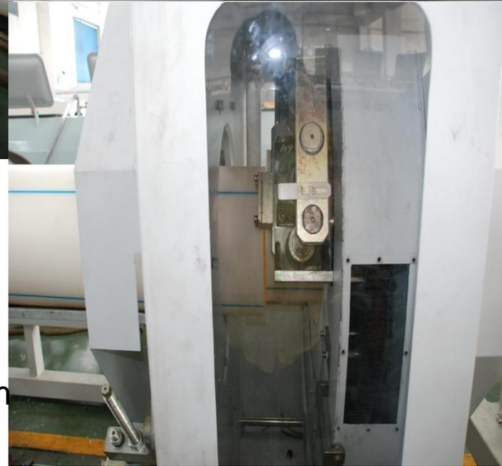
**Type:** Gear transmission、 knife in and out by screw rod、 rotating cutting
