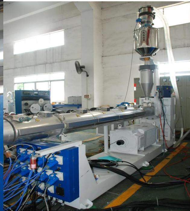
**Main driving motor : 200kw DC motor**
