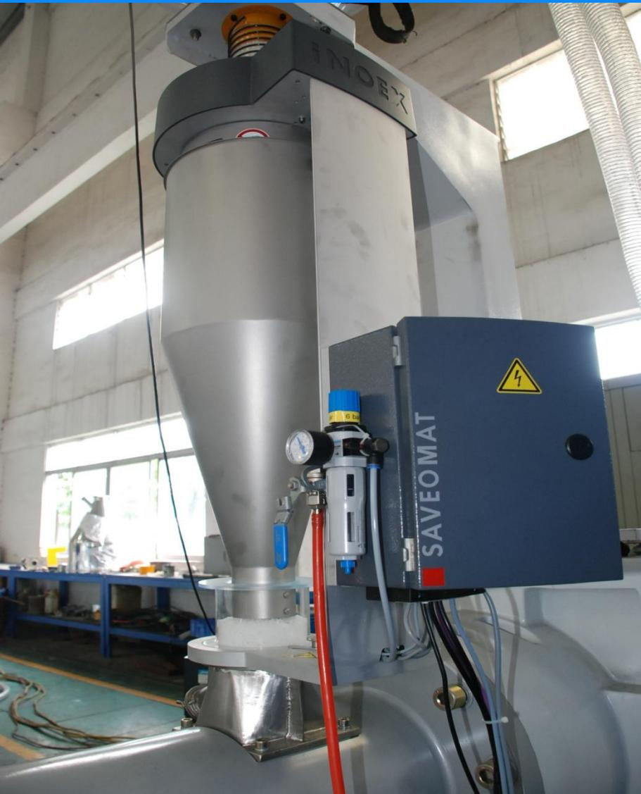
Saveomat IGS.M1 Gravity monitoring system, it is directly **imported from Germany**, the purpose is for better control of thickness of pipes and stable feeding of materials through changing the screw rotate speed and hauling speed.
