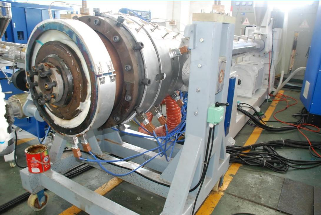
This set of mould has spiral flow channel which ensures an even melt temperature, eliminates melting marks, and overcomes the stripe defect. Mould adopted core thermostat system, greatly reduced blistering, black spots, cracks and other phenomenon which was caused by inner temperature is too high or too low. **W air exhaust device. Fan power 2.2kw .**
