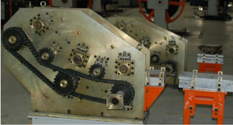
Steel profile preforming
